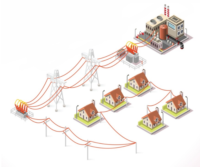
Figure 1. Typical Power Plant with Radial Distribution
