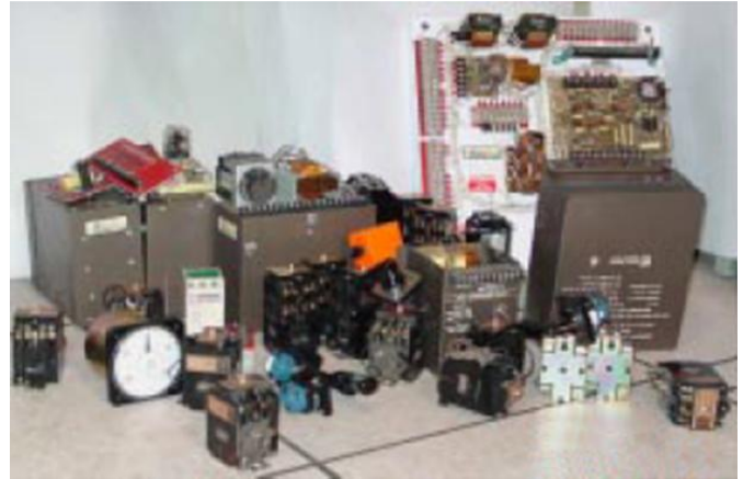
Fig. 4 1970's analog excitation system
