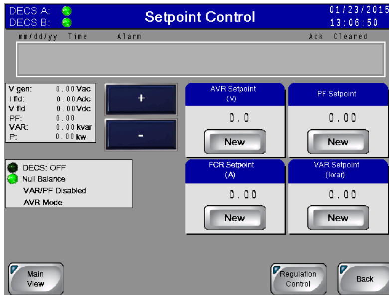
Figure 55. Setpoint Control Screen
