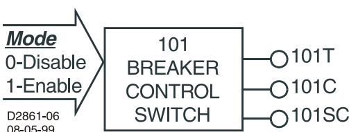
Figure 4-72. Virtual Breaker Control Switch Logic Block
