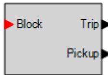
Figure 7-2. Overvoltage Element Logic Block
