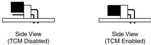
Figure 41-4. Trip Circuit Monitor Enable/Disable Jumper Location
