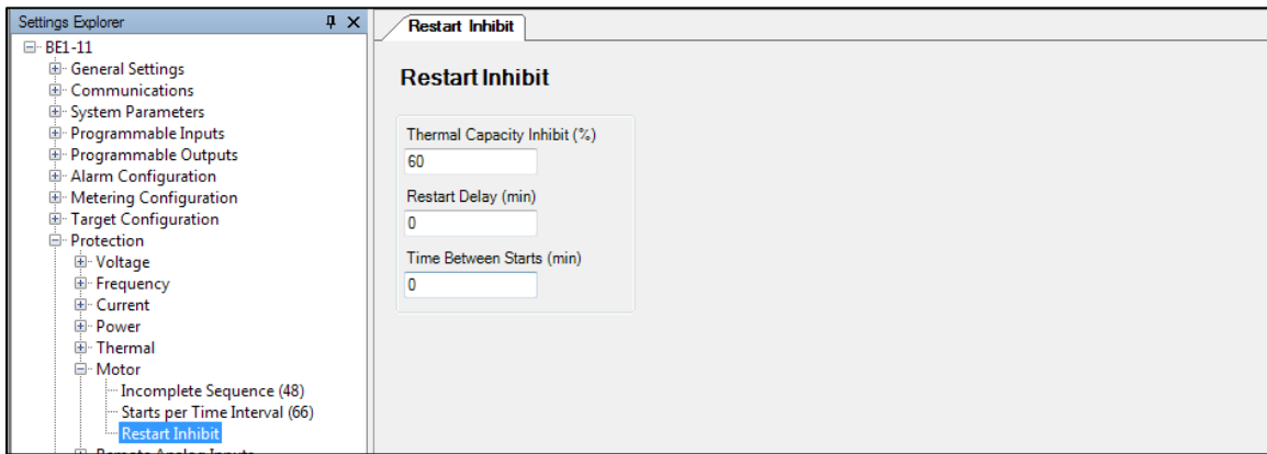
Figure 84-66. Protection, Restart Inhibit Screen
