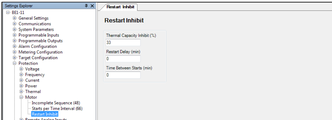
Figure 84-29. Protection, Restart Inhibit Screen
