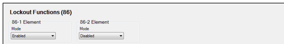
Figure 27-2. Lockout Functions Settings Screen
