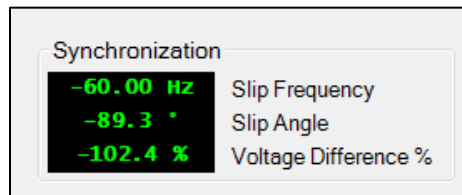
Figure 28-6. Analog Metering, Synchronization Screen
