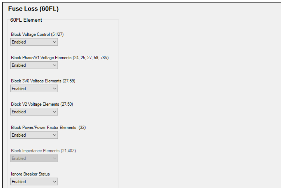
Figure 38-3. Fuse Loss Settings Screen
