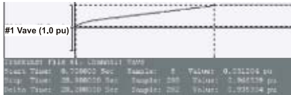
Figure 7: Voltage Softstart Buildup Characteristic
