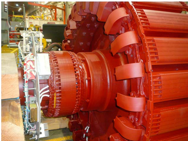
Fig. 5 Brushless Exciter Diode Wheel Assembly
