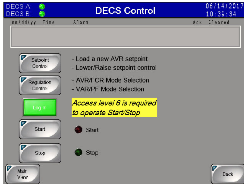
Figure 5-22. DECS Control Screen
