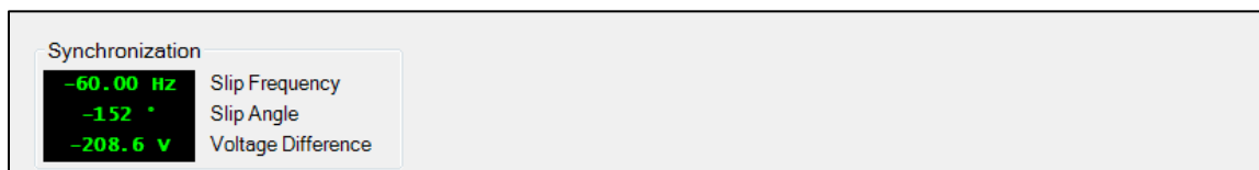
Figure 11-8. Synchronization Primary-Values Metering
