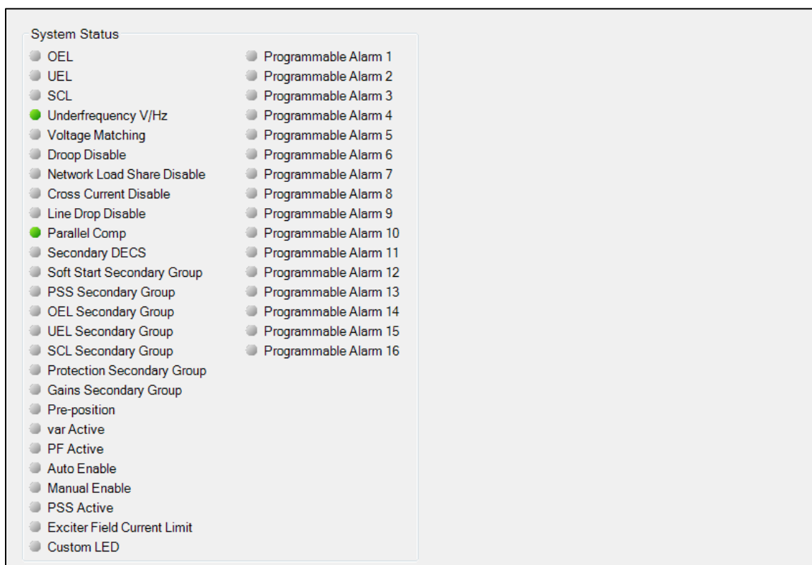
Figure 11-13. System Status Indication Screen
